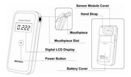
The AlcoScan Model AL7000 analyzes a breath sample to detect alcohol in the lungs.
